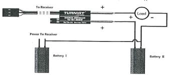
**Note:** this picture show when you have two or more than two battery (Power supplier), you need make **THEIR GROUND CONNECTED** (common ground). Other wise, the Electronic Switch not working.
